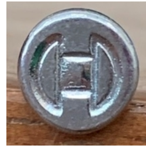
FIGURE 4—BOSCH FASTENER HEAD MARKING
