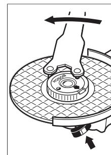
If the quick-clamping nut has been attached correctly and is not damaged, you can loosen it by hand by turning the knurled ring anticlockwise. If the quick-clamping nut is stuck, do not attempt to loosen it with pliers – always use the two-pin spanner. Position the two-pin spanner as shown in the figure.
