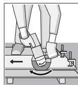
The power tool must always work in an up-grinding motion. Otherwise there is a risk that it will be pushed **uncontrolled** out of the cut. For best results when cutting profiles and rectangular tubing, start at the smallest cross section.
