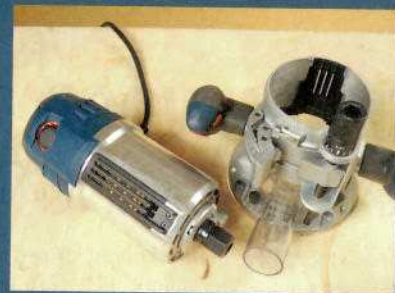
The sliding power contacts it relies on
