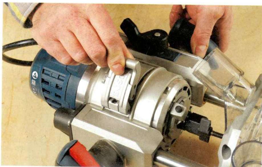
Undoing the lock to remove the motor can
