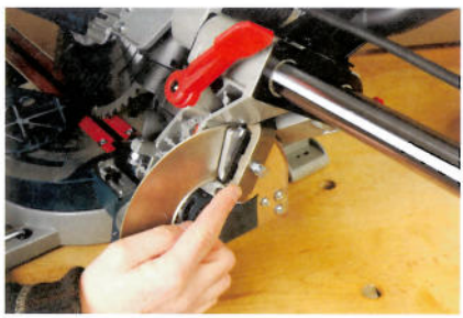
The cam lock lever that allows bevel cuts to be made can be tensioned to make setting very easy
