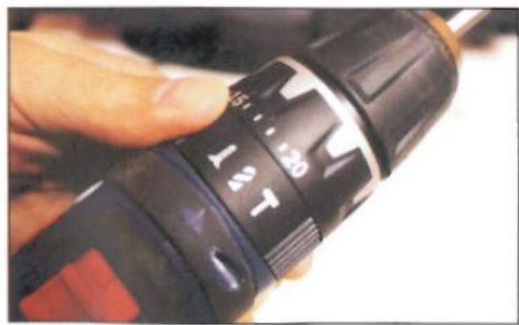
The dual collar lets you shift between torque and drill functions with ease
