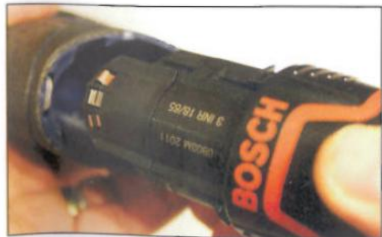
The batteries have overload protection and slot into the handle
