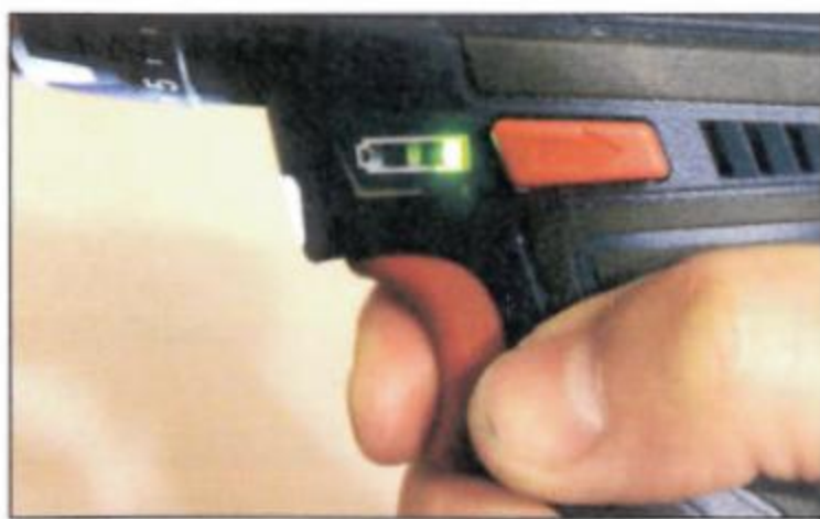
A squeeze of the trigger illuminates an indicator showing the remaining battery power
