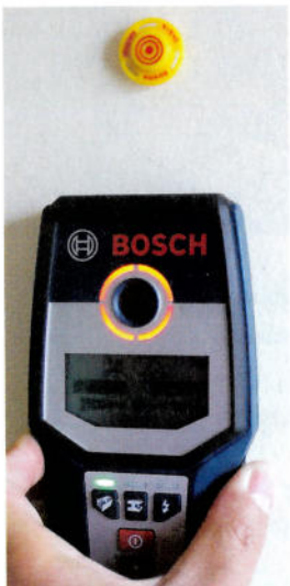
▲ Checking for studs with a known centreline proved perfect. You can mark through the centre hole
