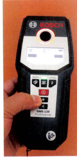
▲ The display can be illuminated and the audio muted with these buttons
