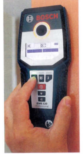
▲ Each function has its own button but they all pick up live cables
