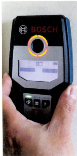
▲ The icon changes to indicate a different problem, in this case a non-ferrous gas pipe
