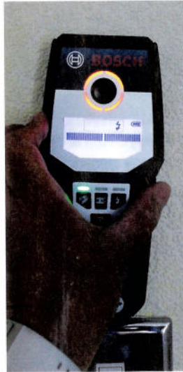
▲ Move near a cable and the ring flashes and the unit beeps loudly
