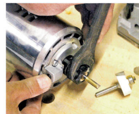
▲ Bit swaps are done with the usual single spanner/spindle-lock configuration
