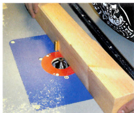
▲ The dual base allows the fixed base to remain in a table
