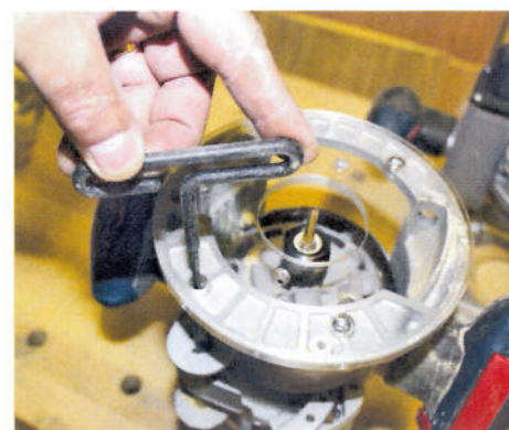
▲ There's a through-the-base adjustment for inverted work
