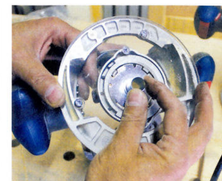
▲ The guide-bush system allows bushes to be swapped in and out without tools
