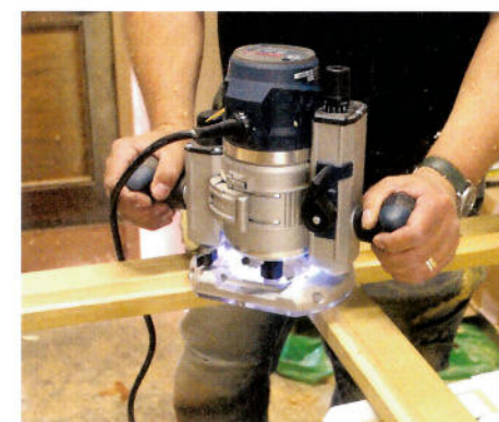
▲ Freehand work is good; although quite big the router is very controllable
