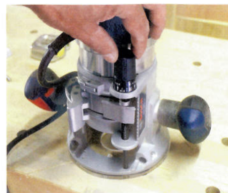
▲ You can also fine tune the cutting depth from above with this knob
