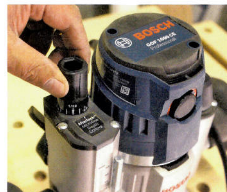
▲ You can fine-adjust the setting even after the plunge is locked
