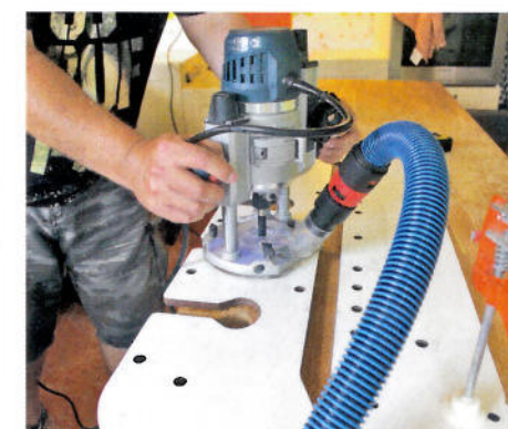
▲ The 1400W motor is man enough for heavy-duty applications such as worktop joints
