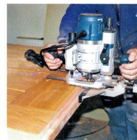
▲ The fine-adjusting fence is great for rebating work
