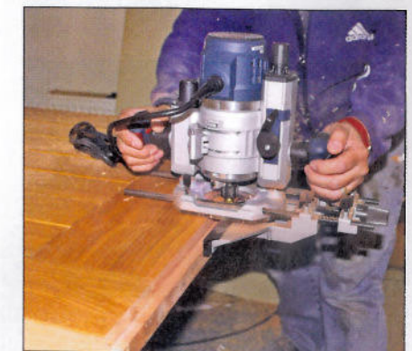
The fine adjusting fence that's supplied with this model is great for rebating work
