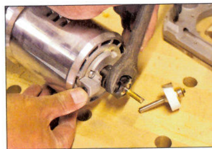
Bit swaps are done with the aid of the usual spanner/spindle lock combination
