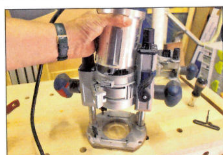
The motor slots into each base very quickly and is locked in place by toggles
