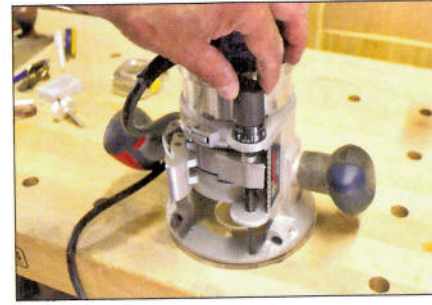
You can fine-tune the cutting depth from above with this knob
