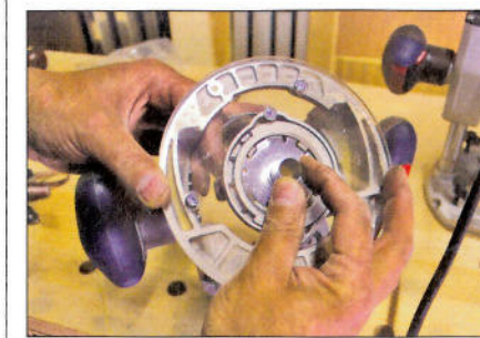
The guide bush system allows bushes to be swapped without tools
