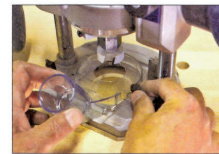
Separate dust adaptors and guards are supplied for each base
