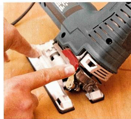
▲ The base tilts and is held firmly once the base angle lever is re-engaged
