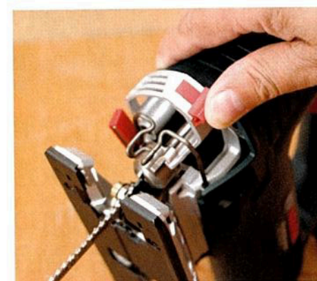
▲ This lever ejects the blade without you having to touch it
