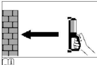
*If the unit was not switched on while being held against the wall, a prompt appears in the display to place the unit against the wall for measuring.*
