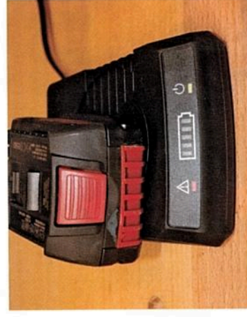
▲ Sit the battery offcentre and the charger shows a red light to indicate that it needs repositioning
