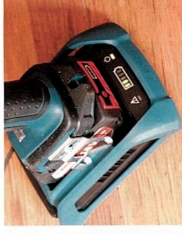
▲ The blue outer cradle allows the battery to slide in and be held securely
