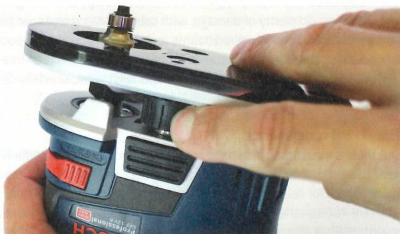
Adjusting the fine tuner, the lock is on the other side
