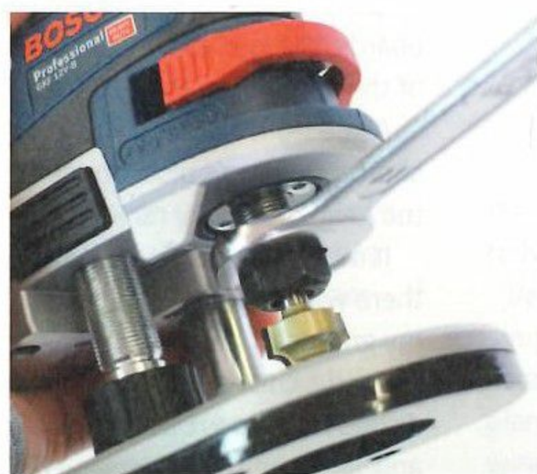
Tightening a bit in the collet
