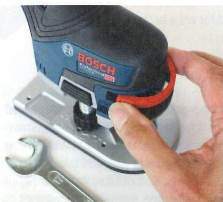
The spindle lock pulls out for bit changes
