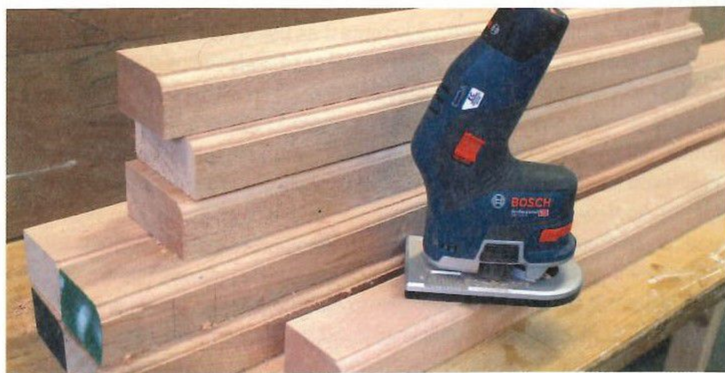
I ran this ovolo moulding with battery to spare
