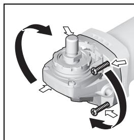
machine head carefully, **without removing it from the housing**, to the new position. Screw in and tighten the four screws again.
