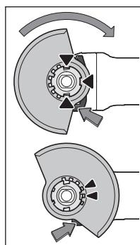
Place the protection guard 7 on the power tool's holding fixture until the protection guard's coding lugs line up with the holding fixture. When doing so, press and hold the unlocking lever 20. Press the protection guard 7 onto the spindle collar until the shoulder of the protection guard is seated against the flange of the machine, and turn the protection guard until it can clearly be heard to engage.
