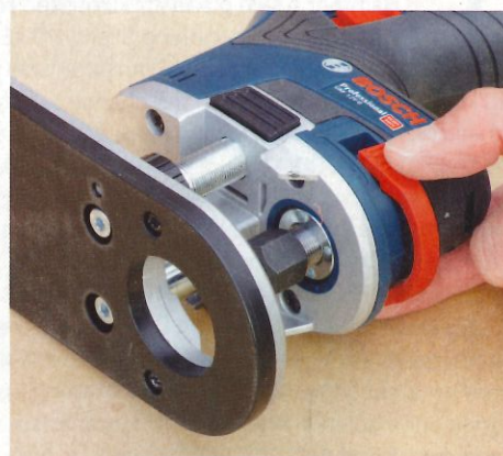
Fitting a bit is a cinch – you pull the red plastic collar (attached to a steel lever) outwards from the body to lock the spindle
