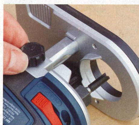
Around the other side of the tool is a thumbwheel for locking the selected depth
