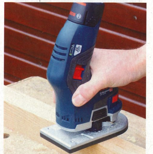
Designed to be held halfway down the tool, your hand naturally rests on the rubber-shrouded ledge, with thumb and fingers wrapping around the body
