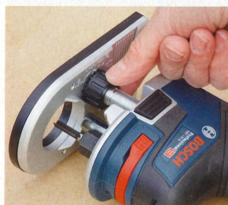
One column is threaded and incorporates a fine adjuster collar at the bottom
