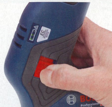
The on/off slider switch is nicely recessed to reduce the chance of accidental activation
