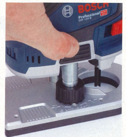
With maximum plunge of 26mm, you can set cutter depth approximately by depressing a large side button
