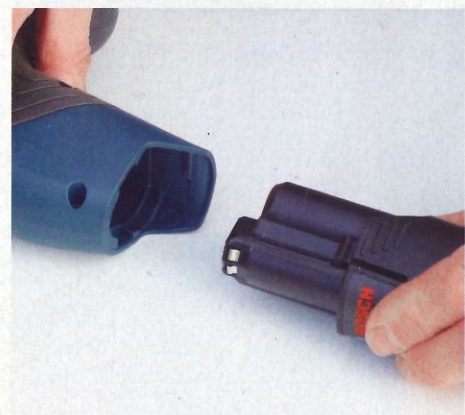
You insert a battery into the top of the tool, with green LEDs illuminating for a few seconds on the plastic casing to indicate remaining capacity
