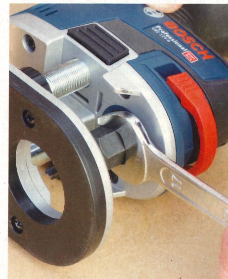
Insert the shank, tighten with the wrench provided and push the collar home again
