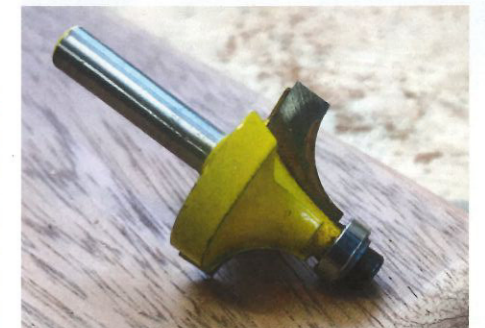
A 9.6mm radius cutter is on the limit but quite possible
