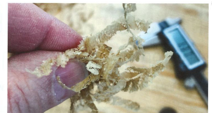
Thick, wide shavings could block the exhaust when used with the extraction bag
