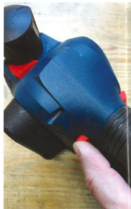
The trigger has a safety switch that can be operated from both sides of the machine
