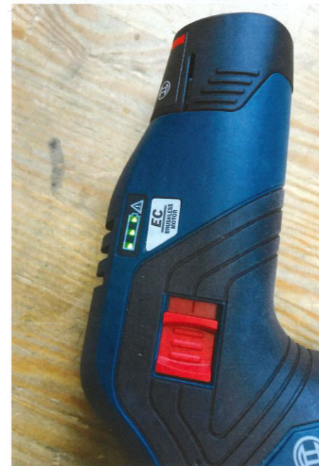
Power levels are recorded in a neat little LED display
