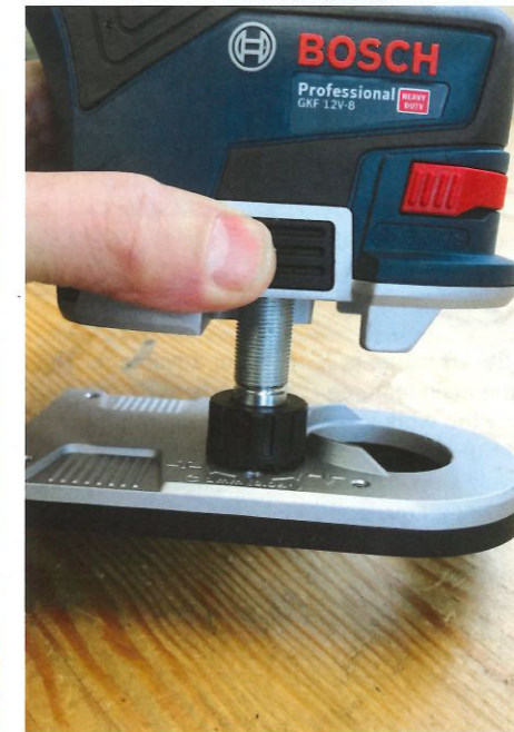
A quick release button makes cutter changes easier
