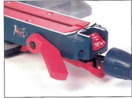
**9** A large lever on the left-hand side then locks the setting securely in place
