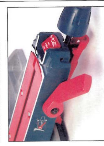
9 A large lever on the left-hand side then locks the setting securely in place
