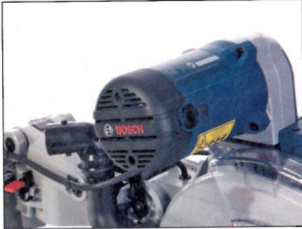
**14** The powerful 2000W brush motor is mounted high up on the machine
