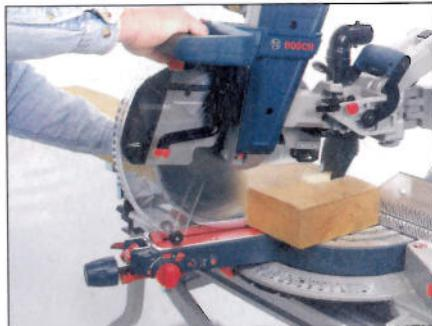
**19** The saw will happily cut material up to a maximum of 104mm thick
