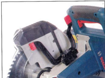
**13** A paddle on the handle releases the guard, which flips back automatically
