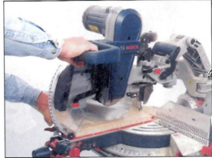
**20** The maximum crosscut capacity at full stretch is a massive 341mm
