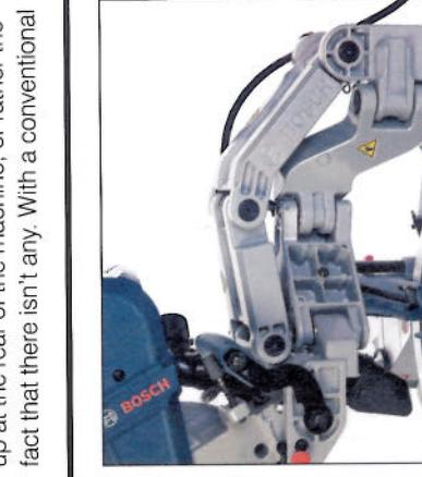
2 ...which does away with the need for any clearance space behind the saw
